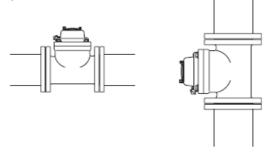
Water meters should always be fitted with a minimum of 3x pipe diameter upstream.
